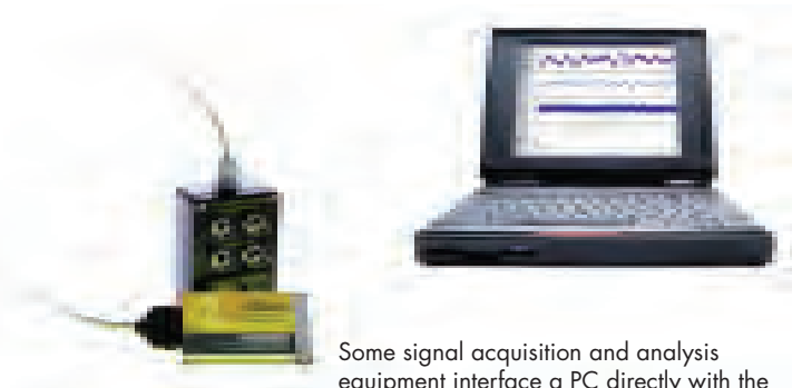
Typical Vibration Analyzer – Note liquid crystal display providing actual vibration waveform information in addition to machine condition analytical capabilities.
